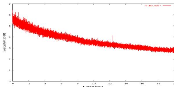
Figure 2. Luminosity/ $10^{34}$   $\text{cm}^{-2}\text{s}^{-1}$  vs. number of turns/1000.
