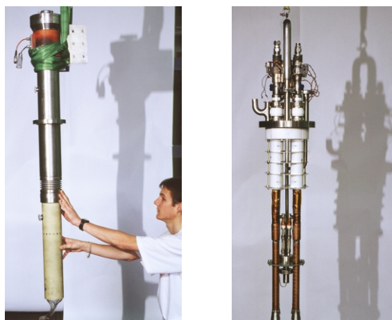
Figure 5: 13000 A prototype and 4x600 A leads assembly
