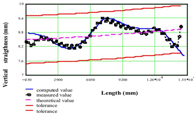
Figure 3 b: The straightness of the MBP2N2 prototype
