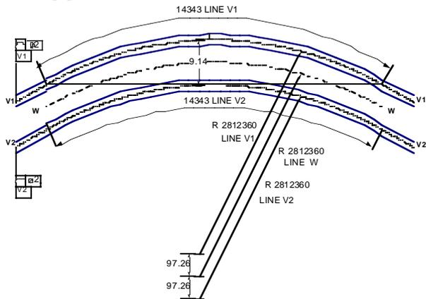
Figure 1: Horizontal theoretical shape of the cold mass in assembling conditions
