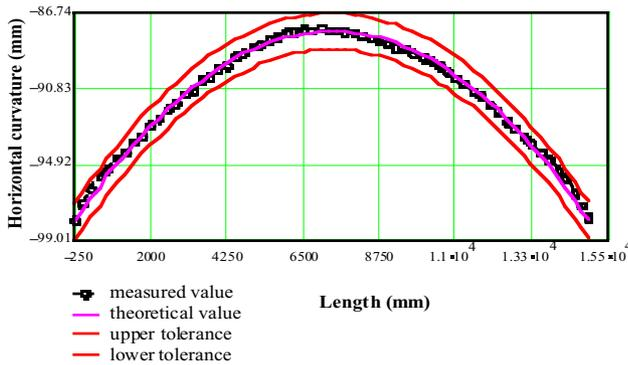
Figure 3 a: The curvature of the MBP2N2 prototype
