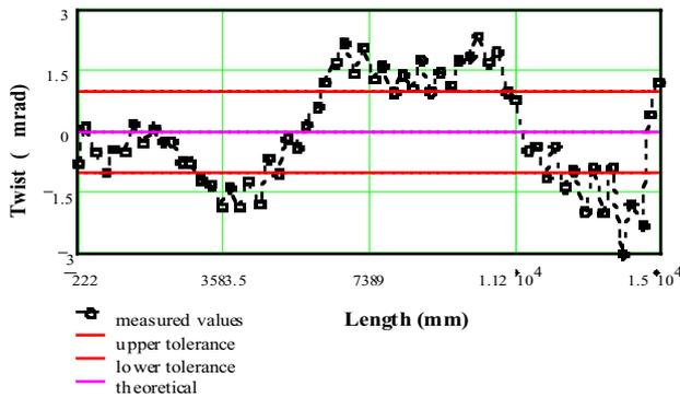
Figure 3 c: The twist of the MBP2N2 prototype
