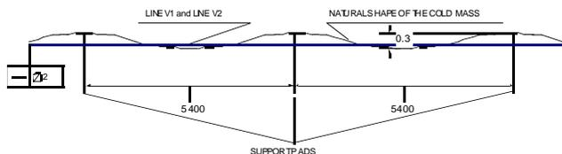
Figure 2: Vertical theoretical shape of the cold mass in nominal supporting conditions (three support pads).
