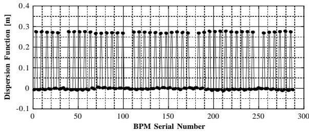
Figure 1: The dispersion function of the SPring-8 storage ring measured by the BPM system.
