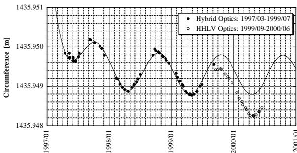
Figure 3: Long term variation of the circumference of the SPring-8 storage ring. The solid line is the expected circumference change from the seasonal temperature variation and the shrinkage of the concrete foundation.
