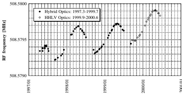
Figure 2: Long term variation of the rf frequency of the SPring-8 storage ring.
