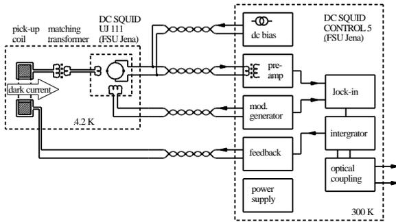
Figure 3: Simplified electrical scheme of the CCC
