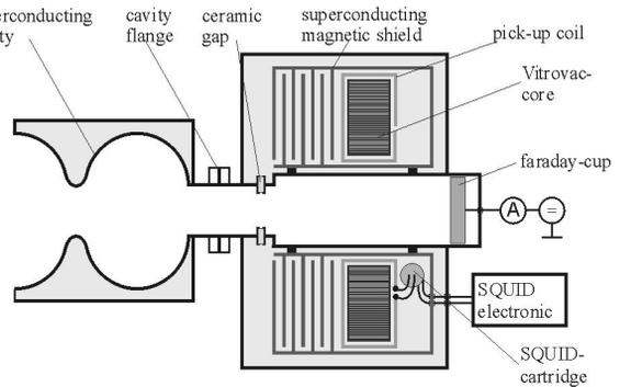
Figure 6: Schematic Design of the CHECHIA CCC
