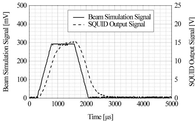
Figure 4: SQUID response and test signal
