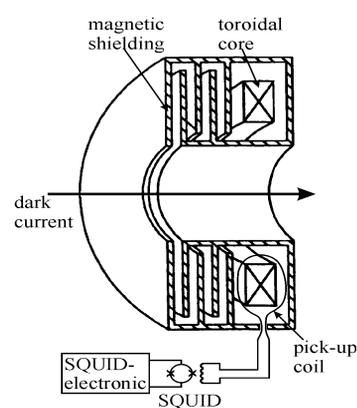
**Figure 2: Schematic view of magnetic shielding, pickup coil and SQUID system**
