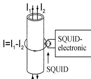
**Fig.1: Principle of the Cryogenic Current Comparator**
