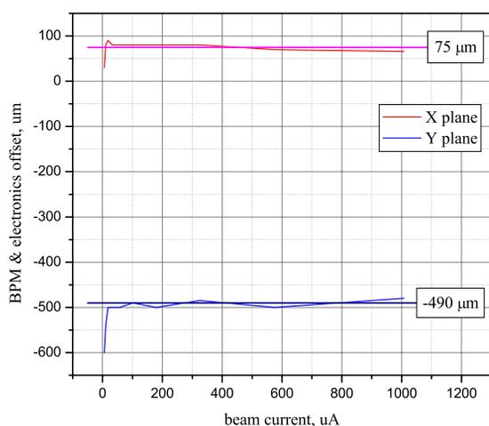
Figure 5: Measured BPM offset.
