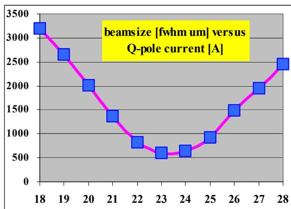
Fig.8: emittance measurements in TL-1.
