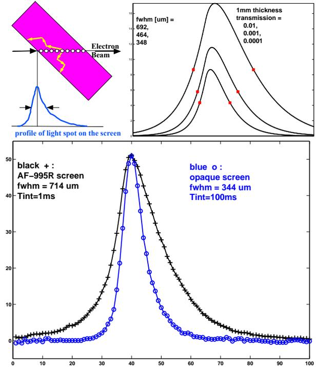
Fig.5: spatial resolution limit due to screen characteristics.
