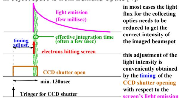
Fig.2: adjustment of light intensity with CCD shutter.
