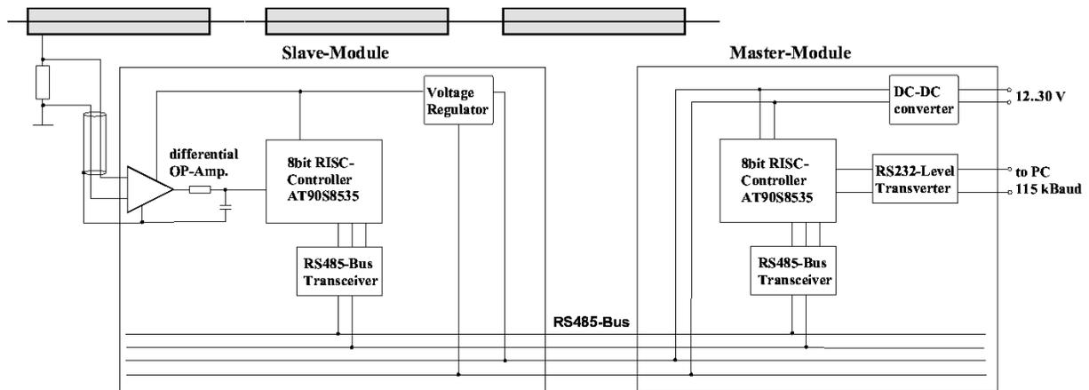
Figure 3: Acquisition electronics for segmented BLM system with longitudinal resolution.
