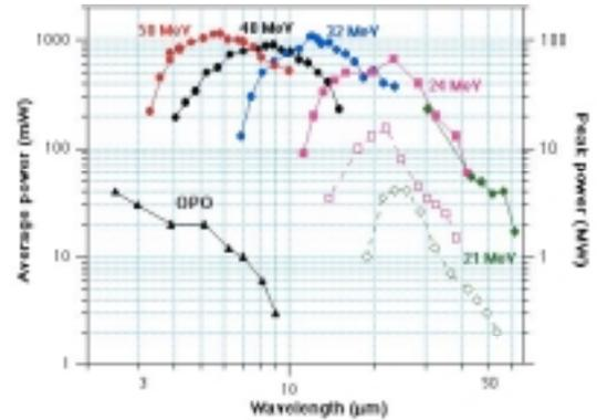
Fig. 7 : Intensity measurement of the CLIO infra-red FEL
