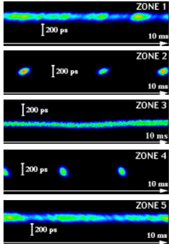
Fig. 10 : Super-ACO FEL pulse measured for different detuning with the double sweep streak camera (Hamamatsu). zone 1 :  $\Delta f_{RF} = -50$  Hz, zone 2 :  $\Delta f_{RF} = -10$  Hz, zone 3 :  $\Delta f_{RF} = 0$  Hz, zone 4 :  $\Delta f_{RF} = +10$  Hz, zone 5 :  $\Delta f_{RF} = +50$  Hz
