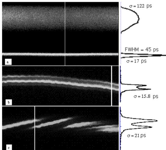
fig. 9 : Example of the Super-ACO FEL (Orsay). Cw FEL (area 3), 1a, Vertical scale = 1.7 ns, Horizontal scale = 1 ms; 1b, 300 ps, 10 ms; 1c, 300 ps, 10 ms; the current,  $I = 50$  mA. The laser temporal distribution with their width RMS, associated to vertical slices for each image, are also plotted.
