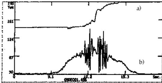
Fig.11: Super-ACO FEL position and intensity versus the difference between the revolution frequency of the electrons in the ring and the round trip time of the photons in the optical resonator.  $I = 90$  mA.
