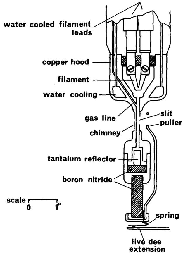
Fig. 3. Hot cathode calutron ion-source
