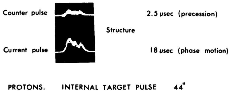
Fig. 7. Time structure of beam striking internal target
