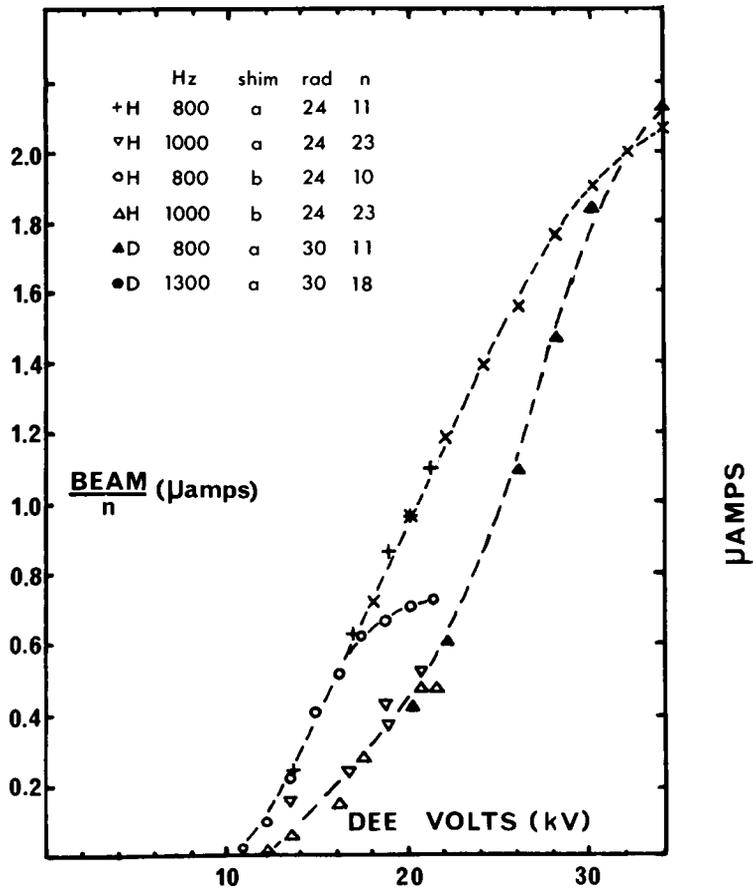
Fig. 6. Variation of internal beam with dee voltage
