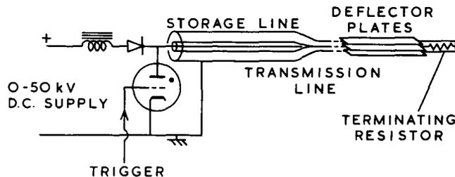
Fig. 11. Time-of-flight beam deflection circuit (schematic)
