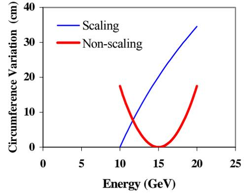
Figure 1: Scaling and non-scaling FFAG orbit patterns (above), and circumference variation with energy (below).
