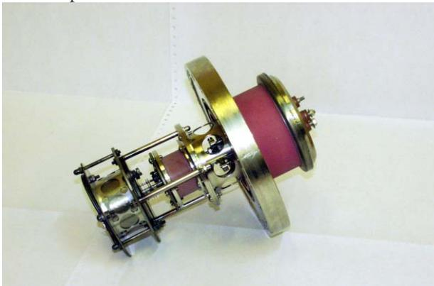
**Figure 1:** Picture of ion source prototype (side view)
