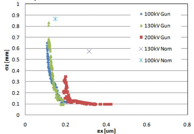
Figure 3: Optimal front for varying gun voltage using the present injector layout.
