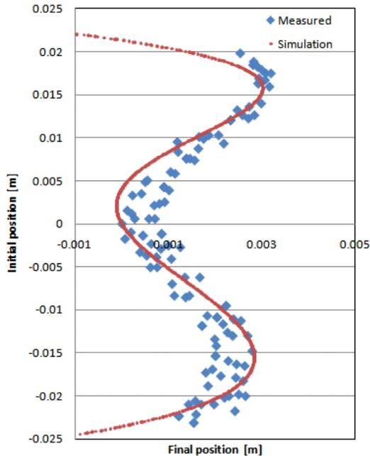
Figure 2: Arrival position of the electron bunch (0.2pC) as a function of initial longitudinal position.
