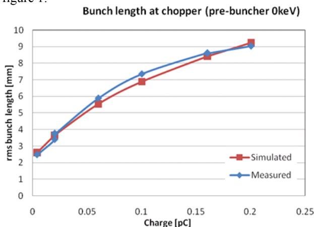
Figure 1: Comparison of bunch length, measured using the beam chopper, with simulation.
