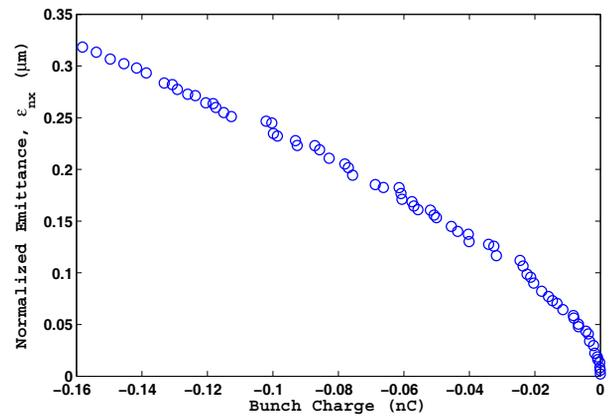
Figure 2: Full-beamline emittance optimization for varied bunch charges.
