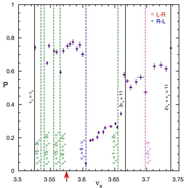
Figure 3: Polarization normalized to the LEP asymmetry plotted vs.  $\nu_x$ . The horizontal bars show the combined slow  $\nu_x$  ramps. The calculated positions are indicated by dashed lines for each spin resonance, and by solid lines for each beam-blow-up resonance. Arrow shows  $\nu_x$  at injection.
