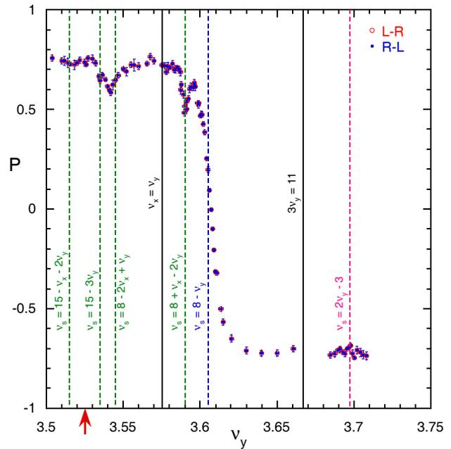
Figure 2: Polarization normalized to the LEP asymmetry plotted vs.  $\nu_y$ . The horizontal bars show the combined slow  $\nu_y$  ramps. The calculated positions are indicated by dashed lines for each spin resonance, and by solid lines for each beam-blow-up resonance. Arrow shows  $\nu_y$  at injection.
