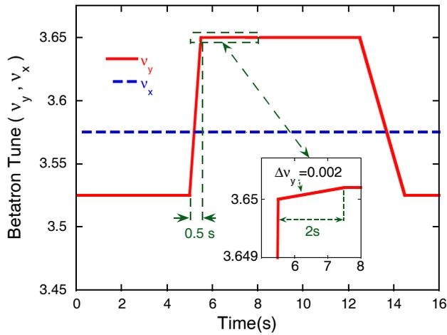
Figure 1: Typical  $\nu_y$  betatron tune ramp during COSY cycle.
