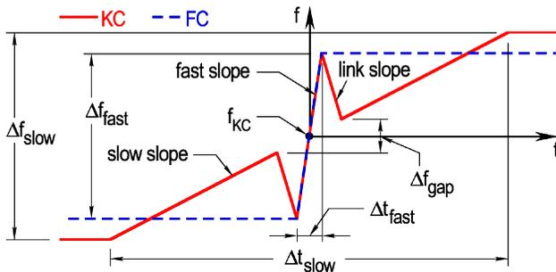
Figure 6: Kondratenko Crossing (KC) [solid line] and Fast Crossing (FC) [dashed line] patterns defining the parameters  $\Delta f_{fast}$ ,  $\Delta t_{fast}$ ,  $\Delta f_{slow}$ , and  $\Delta t_{slow}$ . The KC and FC patterns are both centered at  $f_{KC}$ .
