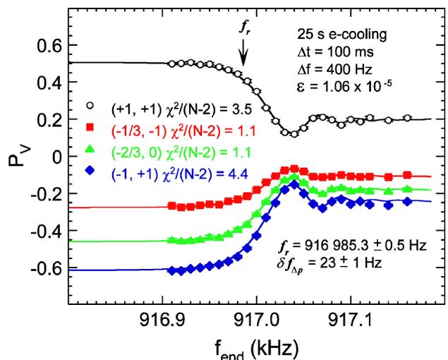
Figure 5: Measured deuteron vector polarizations plotted vs  $f_{end}$  as in Fig. 4. Electron cooling was on for 25 s. The corresponding Chao formalism fit results are indicated in the plot.
