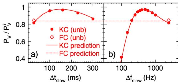
Figure 10: (a) Measured 1.85 GeV/c deuteron  $P_V/P_V^i$  plotted vs slow frequency ramp time  $\Delta t_{slow}$ . (b) Measured 1.85 GeV/c deuteron  $P_V/P_V^i$  plotted vs slow frequency ramp range  $\Delta f_{slow}$ .
