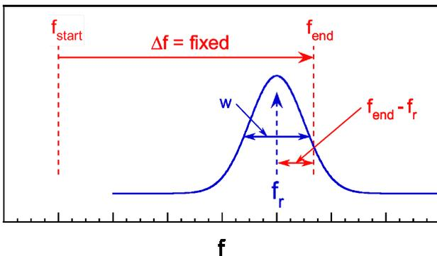
Figure 3: Schematic of the Chao formalism test. The rf solenoid's frequency  $f_{rf}$  was ramped, by a fixed range  $\Delta f$ , for different distances between the ramp's end frequency  $f_{end}$  and the resonance's center  $f_r$ . The curve shows the resonance with a total (FWHM) width  $w$ .
