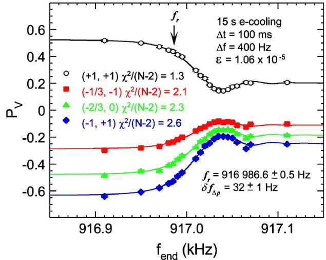
Figure 4: Measured 1.85 GeV/c deuteron vector polarizations plotted vs rf-solenoid end frequency  $f_{end}$ . Its ramp time  $\Delta t$  was 100 ms; its frequency range  $\Delta f$  was 400 Hz, and its  $\mathcal{E}$  was  $1.06 \times 10^{-5}$ . Electron cooling was on for 15 s. The curves are the Chao formalism fits giving the values of the resonance frequency  $f_r$  and of the Gaussian  $\delta f_{\Delta p}$  indicated in the plot.
