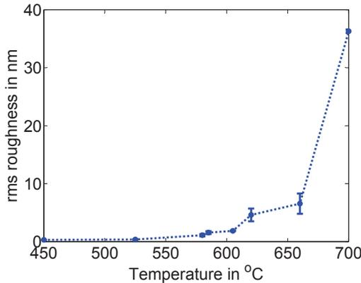
Figure 2: Surface roughness of GaAs vs. temperature.
