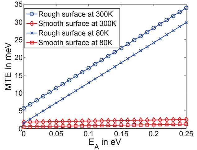
Figure 3: MTE in the slope effect limit vs.  $E_A$  for surfaces shown in Fig. 1 at different temperatures.
