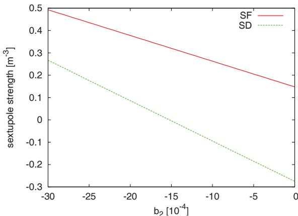
Figure 4: Required sextupole strength for correction of the machine chromaticity vs. dipole error  $b_2$ .
