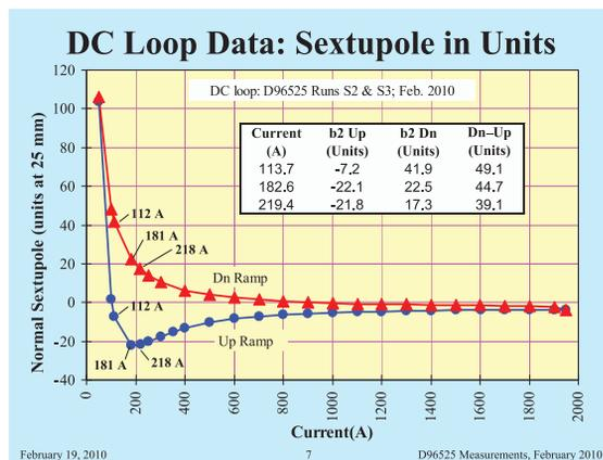
Figure 2: Measured sextupole component  $b_2$  in a spare RHIC dipole. The tabulated currents correspond to  $\sqrt{s} = 5$  GeV, 7.7 GeV, and 11.5 GeV, respectively.
