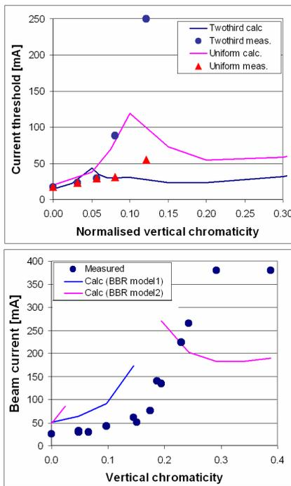
Figure 5: Calculated vertical multibunch threshold versus chromaticity in comparison with measurement. Upper: Diamond. Lower: SOLEIL. The filling pattern is  $\frac{3}{4}$  filling for SOLEIL. See text for the conditions of calculations.
