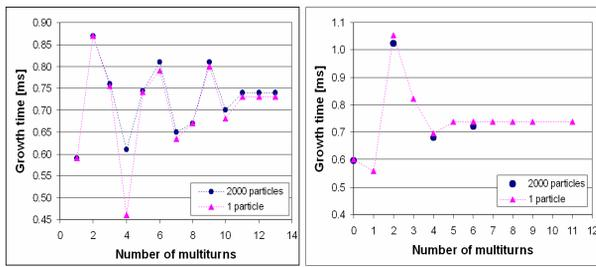
Figure 4: Calculated growth time as a function of turns to which, decaying wakes are retained. Left: SOLEIL. Right: Diamond. With the chromaticity set to zero, the results are verified to be nearly identical between 2000 particles per bunch and 1 particle per bunch cases.
