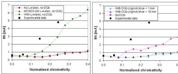
Figure 2: Measured (black squares) and calculated vertical thresholds versus chromaticity in Diamond. See text for the conditions of calculations.
