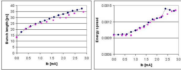
Figure 1: Bunch lengthening (left) and energy spread widening (right) calculated with *sbtrack* (circles), in comparison with measurement (squares) in Diamond. See text for the impedance used.
