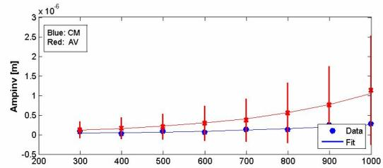
Figure 3: Invariants of the betatron motion averaged over macro-particles and bunches, versus number of turns. Computation assumes 2/3 filling at 300 mA in Diamond with normalised chromaticity of 0.3. See text for the meaning of the two curves.
