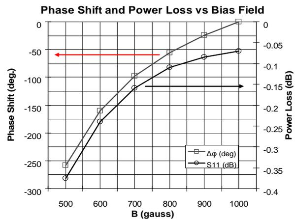
Figure 2: Power loss and phase shift diagram of the phase shifter. 110 mm x 36 mm ferrite-loaded waveguide.
