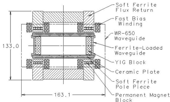
Figure 1: Design concept of a fast phase shifter.
