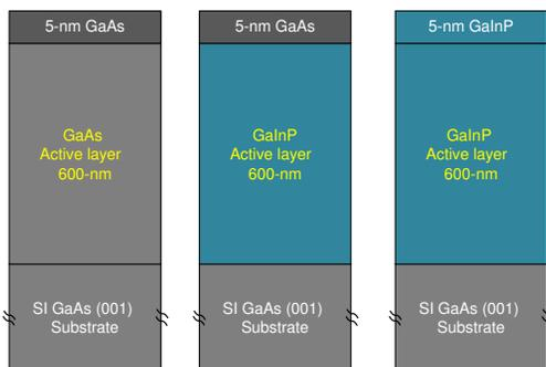
Figure 1: Structure of MOVPE grown samples. For all samples the 5 nm cap layer is p-doped with Zn to a concentration of  $6 \times 10^{19} \text{ cm}^{-3}$  and the 600 nm active layer is doped to a concentration of  $1.5 \times 10^{18} \text{ cm}^{-3}$ .
