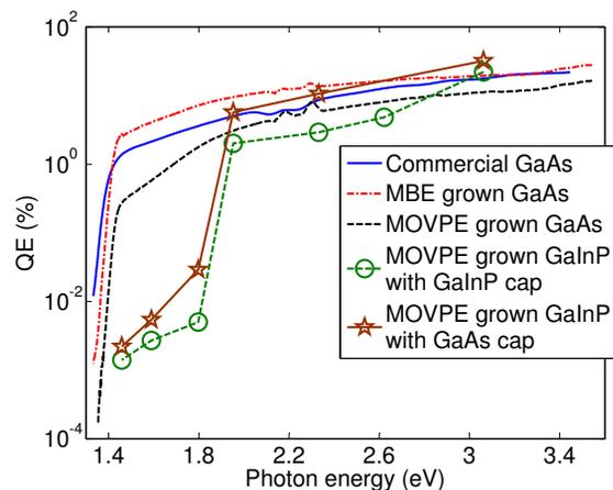
Figure 2: Spectral response of the various samples. The response of the GaAs samples was measured using a monochromator with a Hg vapor lamp, the response of Ga<sub>0.52</sub>In<sub>0.48</sub>P samples was measured using several DC lasers
