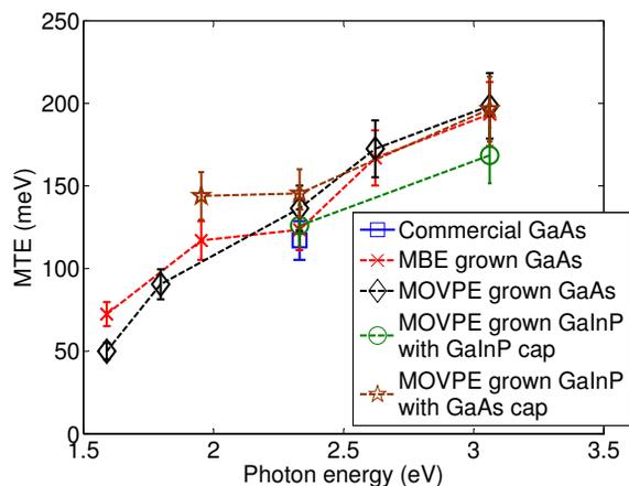
Figure 3: MTE vs incident photon energy. MTE increases as expected with increasing photon energy.
