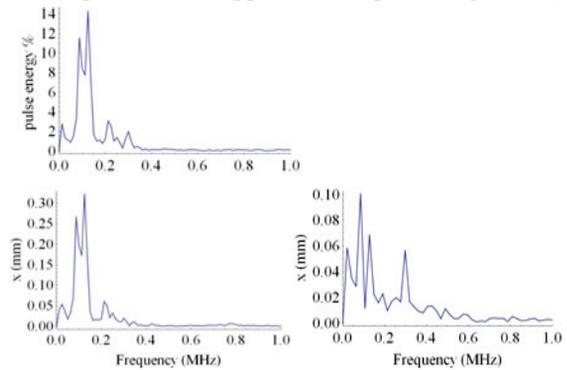
Figure 6: The IR FEL power envelope spectrum (top left), and the horizontal variation spectrum (bottom left). At bottom right is the variation spectrum of the train part before lasing.
