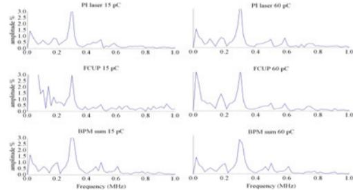
Figure 3: DFT of PD, FC, and BPM signals for bunch charges 15pC and 60pC.
