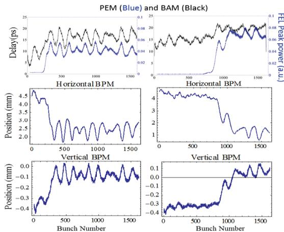
Figure 5: The readings of PEM, BAM, and BPM for two IR FEL power levels.
