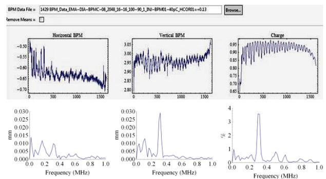
Figure 1: Typical bunch-by-bunch pictures of horizontal and vertical positions (mm), and bunch charge (V) as delivered by a BPM. The spectra are shown in the lower row.
