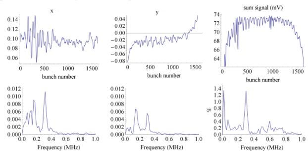
Figure 4: The ‘bunch-to-bunch’ PI laser spot position and intensity as produced by the QPD. The spectra are shown in the lower row.
