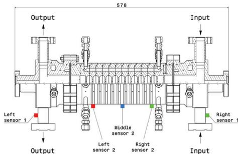
Figure 2: Sensor placement on working system. Sensor 1 shows the sensor position in the first tests and sensor 2 the position in the second tests [1].
