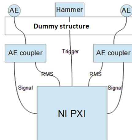
Figure 1: A schematic of the system used for measurements
