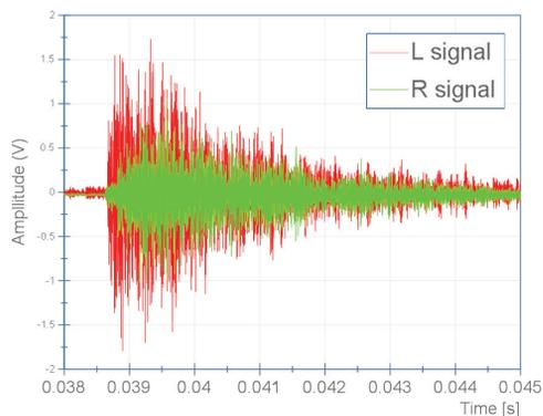
Figure 3: Recorded signal of a BD. Green - acoustic signal of right sensor, Red - acoustic signal on left sensor. The time difference between two signals is detected.
