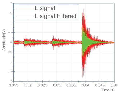
Figure 4: Difference between original and filtered signal. The last peak shows a BD event.
