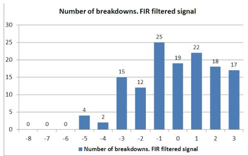
Figure 5: Number of BDs in each cell using FIR filtered signal. Cell number 0 is the cell on which the sensor was placed negative number means that the BD happened toward the input coupler.
