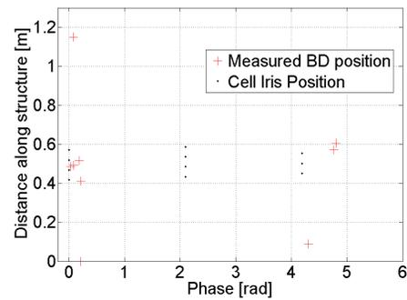
Figure 6: Scatter plot of calculated BD position along structure and phase of the reflected BD signal. The theoretical cell iris position is also shown.
