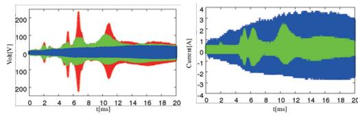
Figure 4: Measured beam induced voltages (left) and currents (right) for 300 kW-equivalent beam. The red, the green and the blue points represent the open, the diodes with 10  $\Omega$  resistors and the 10  $\Omega$  resistors cases, respectively.
