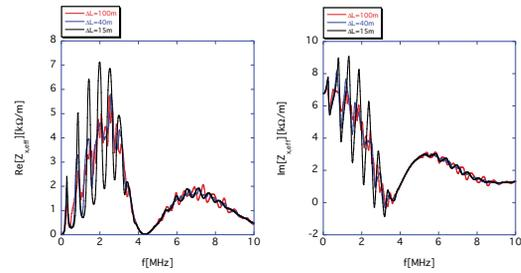
Figure 7: The dependence of the effective one kicker impedance on the difference of cable length, where the diodes with 10  $\Omega$  resistors are connected to the terminals.
