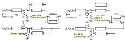
Figure 3: The terminal conditions of kicker cables.
