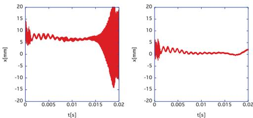
Figure 2: Measurement results of horizontal beam position for 500 kW-equivalent beam. The chromaticity is fully corrected to zero. The left and the right figures show the results for the left and the right kickers in Fig.1, respectively.
