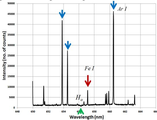
Figure 4: Spectral frame around 656 nm showing Argon spectral lines (blue arrow), an Iron impurity line, and Hydrogen  $H_\alpha$  line in absorption (green arrow).
