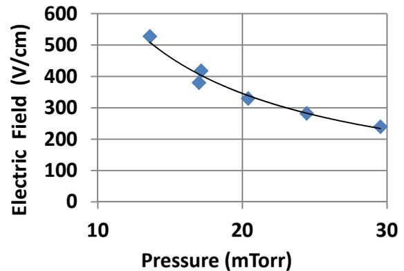
Figure 1: Dependence of breakdown field on pressure for the  $3\pi/5$  mode. Solid line is the hyperbolic fit (power -1).
