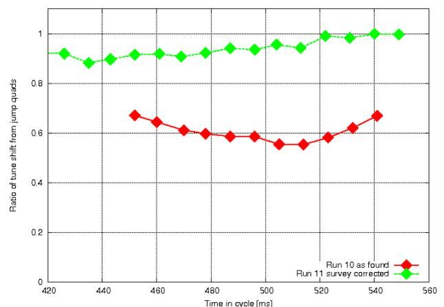
Figure 5: Ratio of the tune shifts measured from equal changes in current in the jump quads, reflecting a significant vertical  $\beta$  function distortion. Red was as measured in Run 10 and green shows a ratio much closer to one after a realignment of several AGS main magnets.
