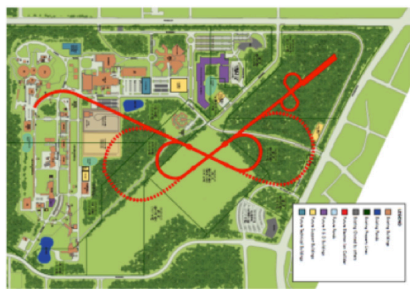
Figure 1: A schematic layout of MEIC (solid red line) and its future energy upgrade (dashed red line) on the JLab site. The ion injector (sources, SRF linac and a compact figure-8 pre-booster synchrotron) is in the upper right corner. The CEBAF linac is on the left with a transfer line to the MEIC electron storage ring.
