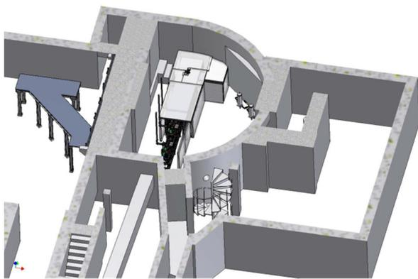
Figure 3: Layout of the CLS Medical Isotope linac.
