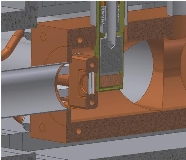
Figure 2: High-power target assembly showing the Ta converter and Mo target holder.
