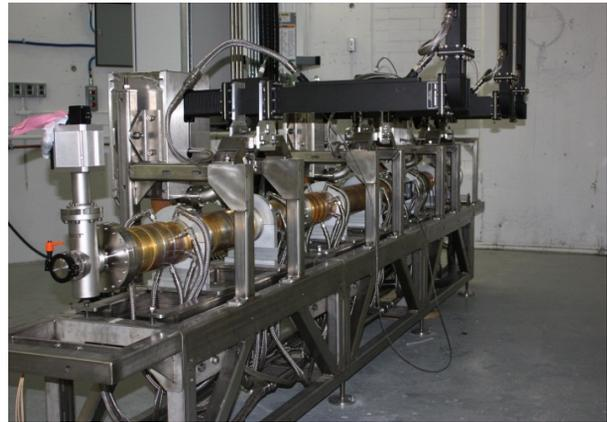
Figure 4: Mevex 35 MeV, 40 kW linac installed at CLS.
