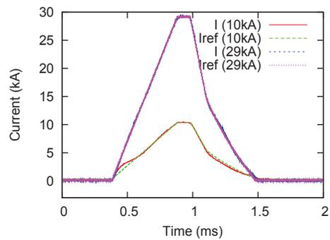
Figure 2: Current pattern of new PBH1 power supply. In case of 29 kA and 10 kA, with reference current pattern and monitoring current.
