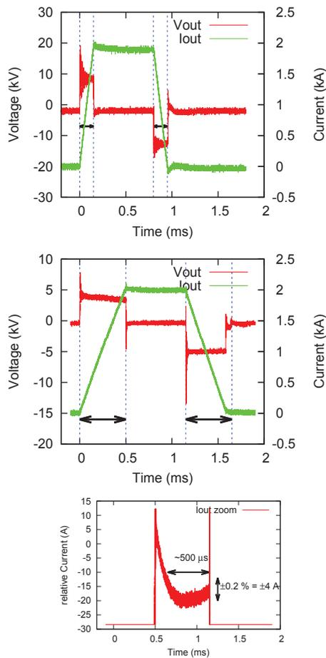
Figure 1: The output current and voltage pattern of new SB PS one bank. The upper is for  $150 \mu\text{s}$  rise/fall, and the lower is for slower rise/fall time ( $500 \mu\text{s}$ ). The bottom one shows good flatness of the current.
