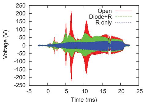
Figure 3: The induced voltage by the beam observed at the kicker power supply with various conditions.
