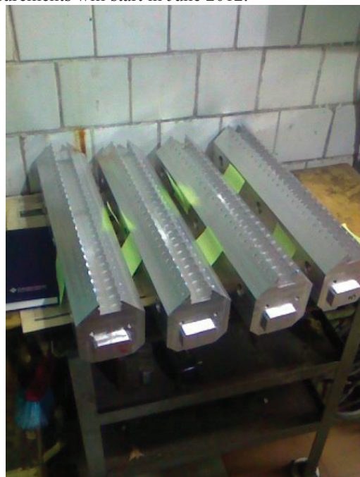
Figure 5: Picture of the magnet holders for the prototype of the helical wiggler.
