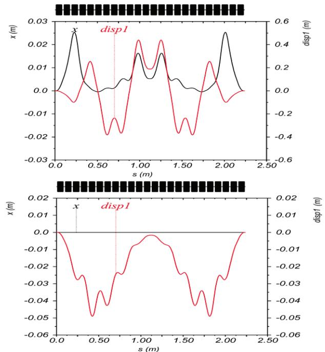
Figure 2: 6 MeV (top) and 12 MeV (bottom) periodic orbits and dispersions of the outward bending super cell.
