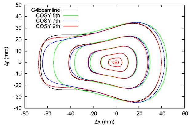
Figure 5: Beam smear due to spherical aberrations after 2 helix periods. G4beamline simulation is compared to various-order COSY Infinity calculations.
