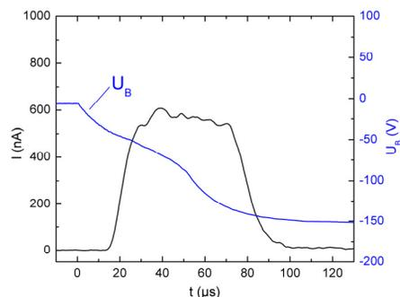
Figure 6: Smoothed voltage switching characteristic of  $U_B$  and the resulting  $C^{4+}$  pulse.
