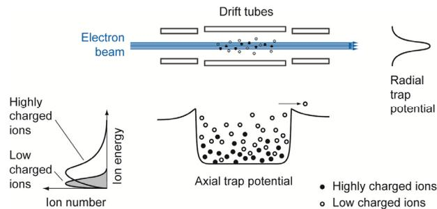
Figure 1: Schematic of ion trapping in the EBIS.
