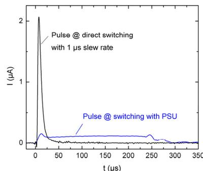
Figure 7: Proton pulses from the Dresden EBIS-A after direct trap opening and after switching with the PSU forming a flat-top pulse shape.
