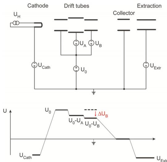
Figure 2: Potential scheme of the Dresden EBIS-A set-up.
