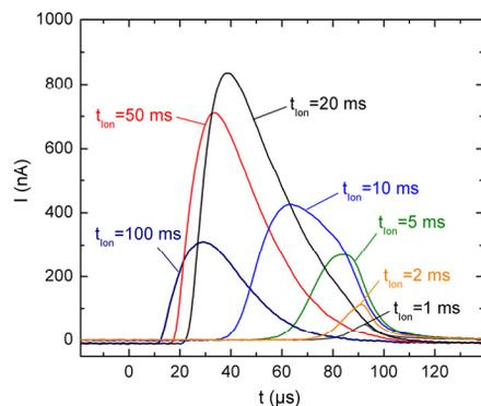
Figure 4: Proton pulses from the Dresden EBIS-A, extracted after different ionization times at a slow rate of 100  $\mu$ s.
