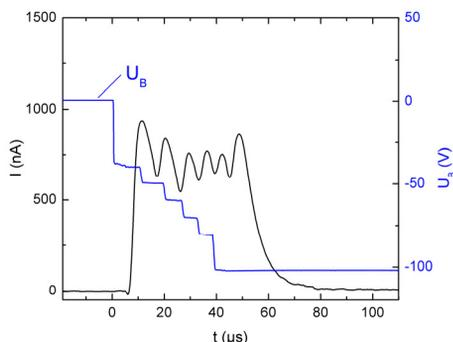
Figure 5: Cascaded voltage switching characteristic of  $U_B$  and resulting  $C^{4+}$  pulse.
