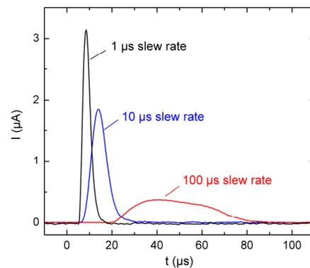
Figure 3:  $\text{C}^{4+}$  pulse extracted from the Dresden EBIS-A, at switching times of  $U_B$  of 1  $\mu\text{s}$ , 10  $\mu\text{s}$  and 100  $\mu\text{s}$ .
