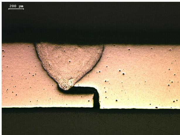
Figure 1: Micrograph of a Be-Be EB weld.
