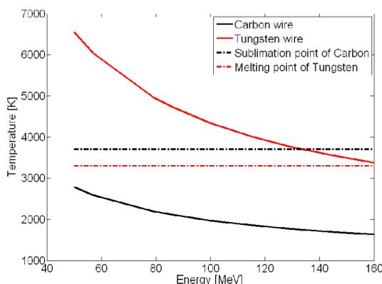
Figure 1: Temperature evolution for 100  $\mu\text{m}$  diameter Carbon and Tungsten wire as function of beam energy, for a LINAC4 40 mA, 400  $\mu\text{s}$  pulse and typical beam sizes at the monitors locations.
