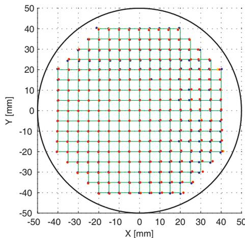
Figure 6: 2D map of the PU response to different wire positions for grounded rings (red), floating rings (orange) and no rings (blue).
