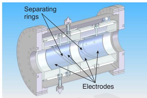
Figure 1: Cross-section view of the beam position monitor.
