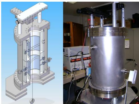
Figure 2: Stretched-wire test setup.
