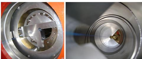
Figure 3: BPM with the alignment components.
