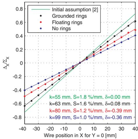
Figure 5: BPM response to wire displacements in X-axis.
