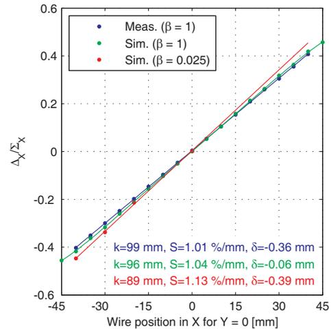
Figure 7: Simulations ( $\beta = 1$  and 0.025) compared with the wire measurements for the BPM with no separating rings.
