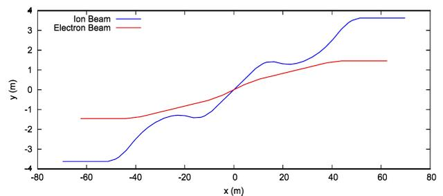
Figure 3: Scaled layout of the electron and ion interaction regions together, produced using MAD-X survey output.
