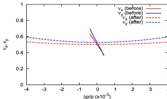
Figure 7: Chromatic dependence of the fractional betatron tunes for the ion ring before and after the sextupole chromaticity compensation.
