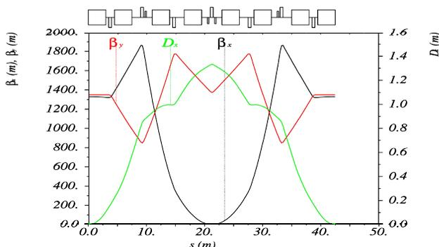
Figure 5: Optics of the ion CCB.
