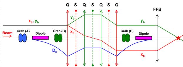
Figure 2: A conceptual drawing of a CCB with an even-symmetry dispersion and an odd-symmetry horizontal betatron trajectory.
