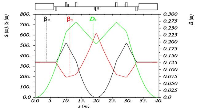
Figure 4: Optics of the electron CCB.
