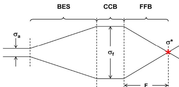
Figure 1: Schematic of the Interaction Region (IR) design consisting of the Beam Extension Section (BES), Chromaticity Compensation Block (CCB), and Final Focusing Block (FFB).
