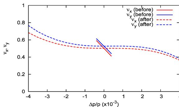
Figure 6: Chromatic dependence of the fractional betatron tunes for the electron ring before and after the sextupole chromaticity compensation.
