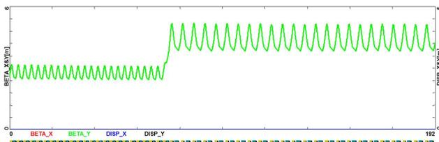
Figure 2: Matched beta functions as calculated by OptiM for the new lattice design.
