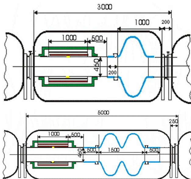
Figure 1: Engineering sketch of the short(top) cryomodule and the intermediate(bottom) cryomodule.
