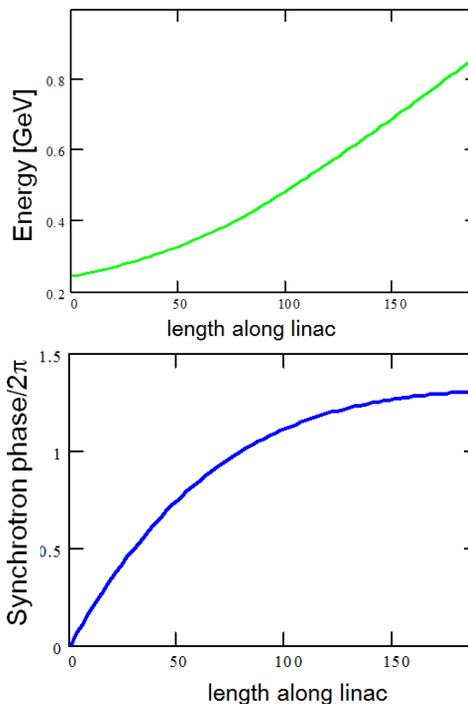
Figure 5: Variation of the beam energy (top) and synchrotron phase (bottom) as a function of length along the linac.
