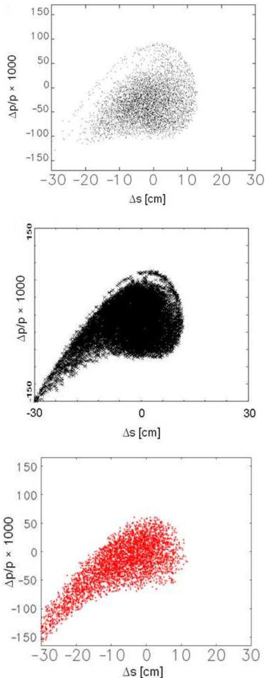
Figure 6: Longitudinal phase space at the end of the linac using  $10^4$  particles tracked with ELEGANT (top), OptiM (middle) and G4beamline (bottom).
