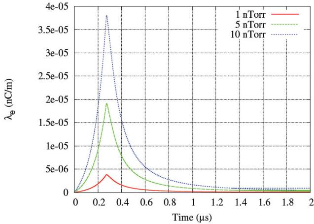
Figure 2: Evolution of electron cloud density with time for 200 consecutive bunches at residual gas pressure 1, 5 and 10 nTorr.
