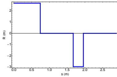
Figure 2: Bending radius as a function of orbit distance for one cell in the arc sections of SuperKEKB positron damping ring.
