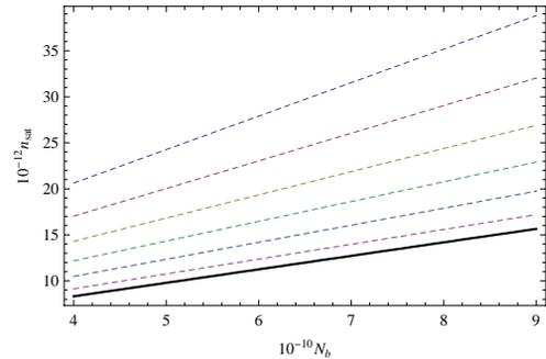
Figure 2: Plot of electronic densities of saturation  $n_{sat}$  vs  $N_b$ , (12) and (13)), withf uniform (solid line) and gaussian (dashed lines) electronic distribution for  $\tilde{a} = 0.04$ ,  $\tilde{r}_0 = 0$ ,  $\tilde{\sigma} = 0.3$  and  $p = 2 \div 3$ .
