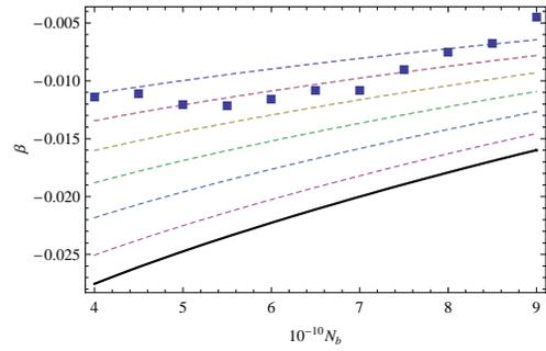
Figure 5: Comparison of the quadratic coefficient  $\beta$  (Eq. (14)) derived using ECLLOUD simulations (points) and using the analysis of previous sections (dashed lines) with  $p = 2 \div 3$ . The solid line is the result by assuming a uniform density.
