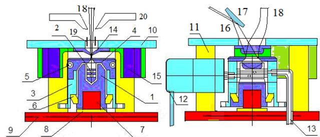
Fig. 3: Schematic of the Advanced version of the Penning discharge SPS for pulsed and CW chopped  $H^+$  beam production.
