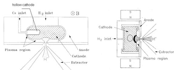
Fig. 1: Advanced version of magnetron with hollow cathode for suppression of discharge noise.
