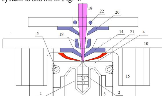
Figure 4: Extraction system of DT SPS
