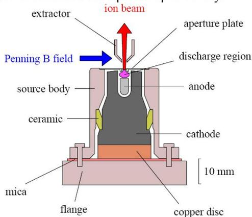
Figure 2: Schematic of ISIS version of Penning discharge SPS [11].
