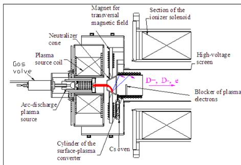
Figure 2: Generation of cold jet of D<sup>-</sup> plasma for resonant charge exchange negative ionization of polarized hydrogen atoms (INR version) [3].
