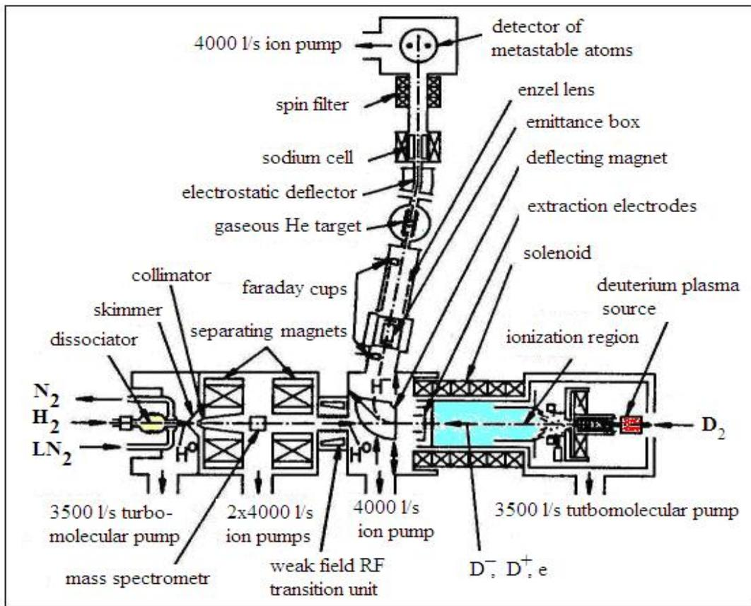
Figure 1: Schematic diagram of atomic beam polarized ion source with resonant charge exchange ionization [5].
