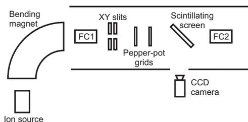
Figure 1: Experimental setup at INFN-LNS.
