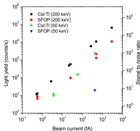
Figure 3: Calibrated light output and signal-to-noise ratio for CsI:Tl and SFOP irradiated with 200 keV and 50 keV proton beams. Note that the beam current was estimated, thus the results may shift “left” or “right” within the uncertainty of one order of magnitude [8].
