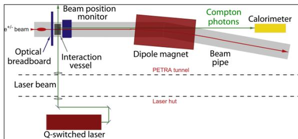
Figure 2: Overview of the laser-wire setup.
