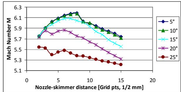
Figure 3: Mach number plotted as a function of nozzle-skimmer distance, with the aperture angle  $\alpha$  as parameter.
