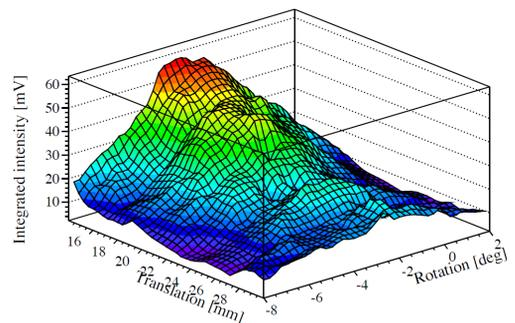
Figure 1: Vertical polarization component of CDR spatial distribution for one target configuration.
