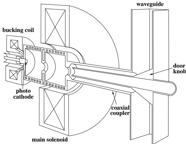
Figure 4: Cross sectional view of the RF gun, showing the one and half cell gun body, the main focusing solenoid and the bucking coil used for imposing the Neumann's boundary condition at the cathode plane for emittance compensation. The RF power is fed through the coaxial line via the waveguide-coaxial line door-knob transition. Due to its cylindrical symmetry, deflecting modes should be suppressed to the minimum.
