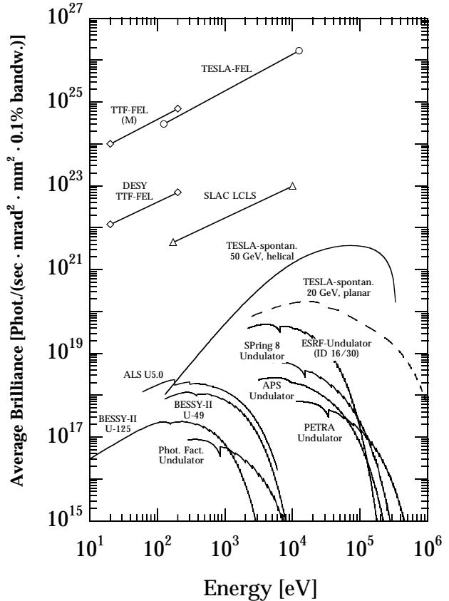
Figure 2: Spectral average brilliance of XFELs and various third generation synchrotron radiation sources
