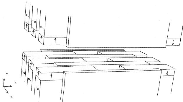
Figure 6: Perspective view of  $1\frac{1}{2}$  periods of the so-called four-magnet focusing undulator (4MFU) which combines dipoles and quadrupoles. They are interlaced with each other. The blocks marked with arrows are permanent magnets. The rest are soft-iron poles.
