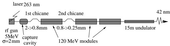
Figure 3: Beamlne layout of the TTF VUV FEL phase I
