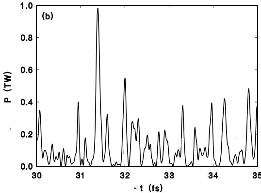
Figure 7: A zoom-in view of the temporal structure of a 180 fs long radiation pulse near the saturation point for a 1 Å FEL. It is simulated with a one-dimensional linear code [22].
