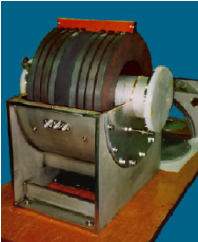
Fig.5. Fabricated untuned RF cavity.
