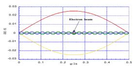
Fig.2. A combination of long wavelength RF and short wavelength RF provide both large energy acceptance and strong focusing.
