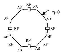
Fig. 1 A schematic of a storage ring with achromatic bends (AB) and RF system (RF) located in dispersion-free straight section. The number of RF systems could be smaller than number of straight sections.
