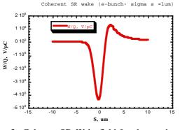
Fig. 3 Coherent SR Wake-field for electron bunch with RMS bunchlength of 1 micron.
