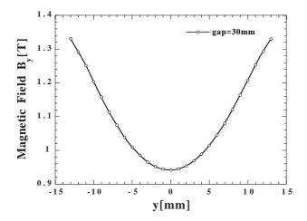
Figure 5: Field distribution of the y-direction in the central pole at the gap of 30 mm.
