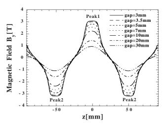
Figure 3: Field distribution along the z-axis at seven different gaps.
