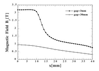
Figure 4: Field distribution of the x-direction in the central pole at two different gaps.
