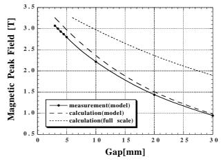
Figure 6: Measured (solid line) and calculated (long- and short-dashed lines) gap dependence of the magnetic peak (Peak1) field.
