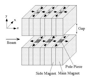
Figure 1: Schematic view of the magnet array of the model multipole wiggler. The arrows on the magnets indicate the directions of the magnetization.
