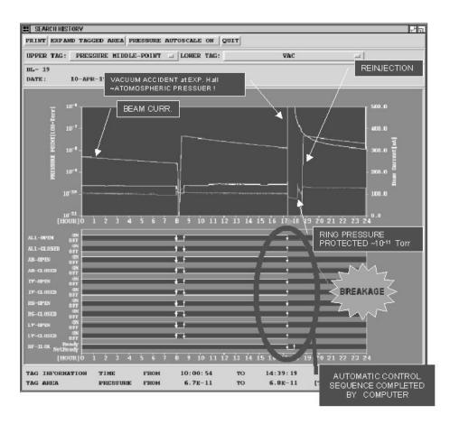
Fig.2 Retrieval result generated by the archiving system to inspect whether two accelerator components are functioning properly.
